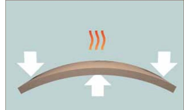
Owing to Resysta's thermoplastic properties, the material can be heated and formed into organic shapes. This offers completely new design options without affecting the highly-desirable tropicalwood look.
