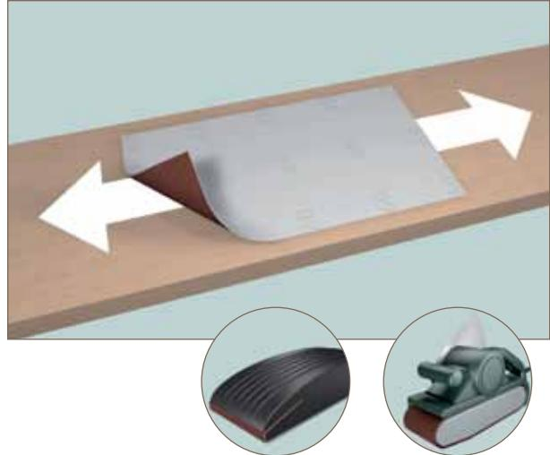
Likewood, Resystashallonlybesandedinlongitudinaldirection. Depending on the surface structure desired, we recommend sandpaper with a grain between 24 to 60. Finer sandpapershallonlybeusedtoremove dirt.
