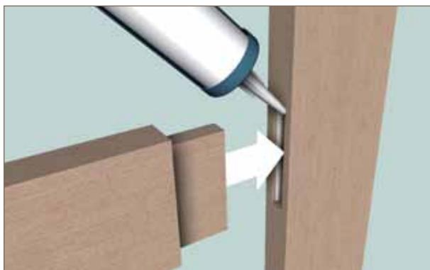
When installing Resysta, standard screws can be used as with wood. Owing to the material's high density, we recommend pre-drilling, before returning in the screws. In almost the same manner, standard nails can be used. Owing to the material's high density, only nails with a certain minimum thickness should be used. Single Resysta profiles can also be connected using hinges or like with wood, tongue and groove (additional bonding recommended).
