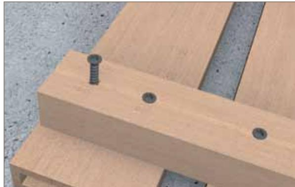
reinforcement – if necessary (increases stability)
