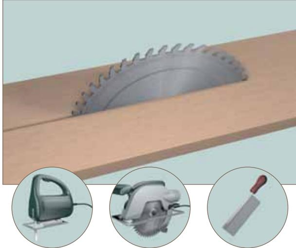
Resystacanbecutinlongitudinalaswellasatransversal direction with all standard saws.
