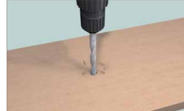
Resystacanalsobeprocessedwithstandardwood drilling machines.
